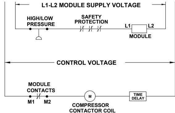
**IMPORTANT:** Bristol recommends a 4-minute delay on break anti-short cycling time delay to prevent contactor chattering.
