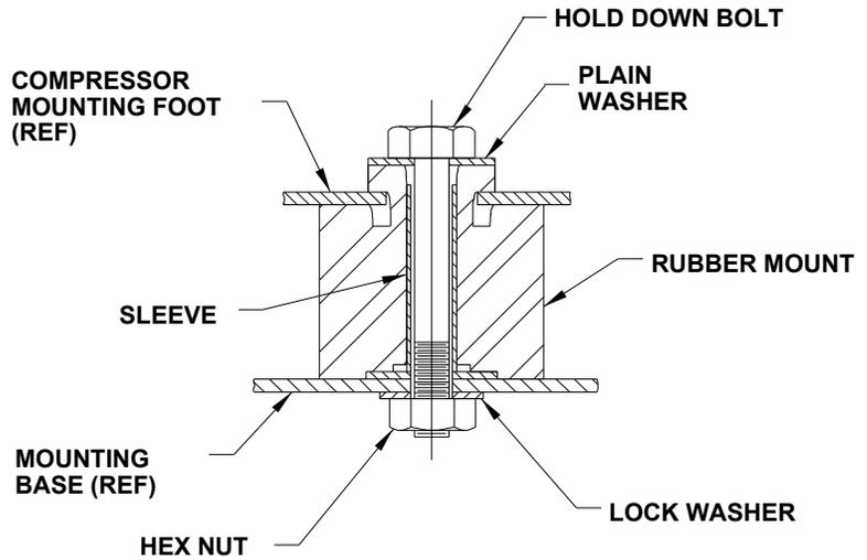
**NOTE: RUBBER MOUNT IS SHOWN IN NON-COMPRESSED FORM. TIGHTEN HOLD DOWN BOLT UNTIL BOTTOMED-OUT AGAINST SLEEVE.**
