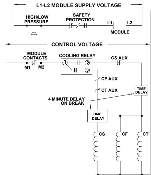
**IMPORTANT:** Bristol recommends a 4-minute delay on break anti-short cycling time delay to prevent contactor chattering.
